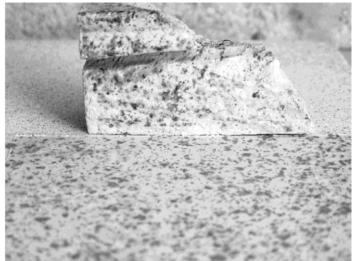
Figure 7: Terra Cotta fragment sits atop a precast panel base-coated with light grey Aquathane UA210 E and top-coated with AquaSpex 220 , incorporating 1500-micron Charcoal Grey flakes. The combination closely matches the original material.
