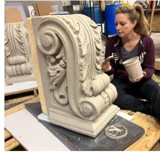
Figure 6: Application of Sil-Quathane 222 to a replacement unit cast with Custom System 45.
