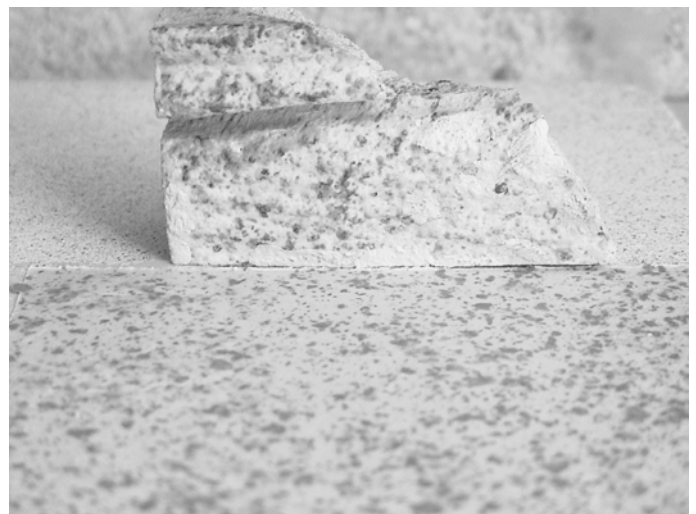
Figure 8: Terra Cotta fragment sits atop a precast concrete panel which has been base-coated with light grey Aquathane UA210 E and top-coated with AquaSpex 220 , incorporating 1500 micron Charcoal Grey flakes. The combination provides a final finish which closely matches the original material.
