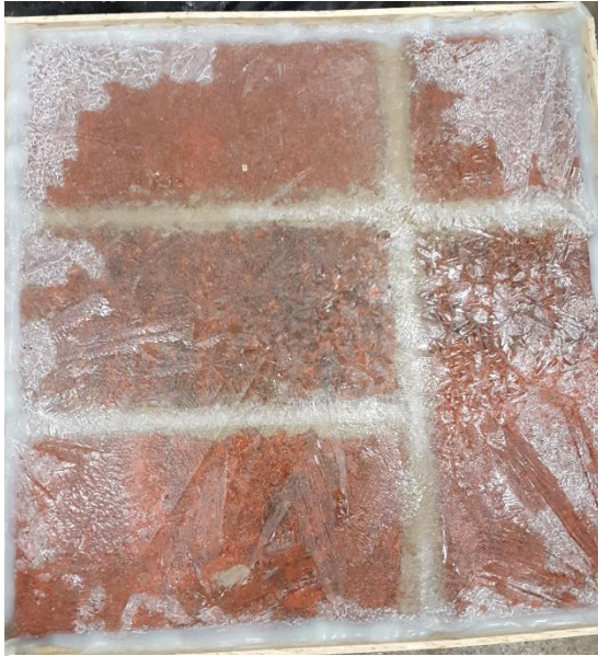
4. Test panels of Rosendale 12M/ICE -9RL "Ultimate Mortar" resisted 50 cycles of freeze-thaw beneath ponded deicing salt solution without damage.
