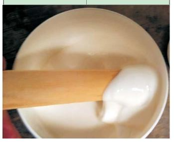
Higher Viscosity = Deeper Penetration = High Durability It may seem counter-intuitive, but SILAN-TREAT 88C's high viscosity actually helps it penetrate better than common silanes because the treatment is held in place long enough to fully penetrate even the densest concretes.
