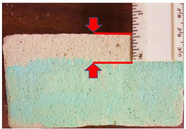
Above represents the penetration depth of *Silan-Treat 88C* into 3000 psi concrete patch, with an average depth of  $\frac{1}{2}$ ". The off white area is where *Silan-Treat 88C* is present and the blue dye could not absorb.
